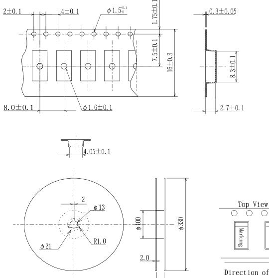
Direction of feed Conforming to EIAJ RC1009B
